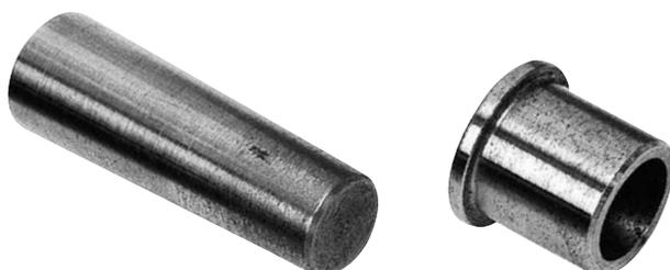
For sealing off leaky condenser and heat exchanger tubes without damaging tube sheets. Tapered pin is driven into ring, which is tapered on the inside and is parallel to tube on the outside. This gives even expansion to the ring and a long contact to the seal.
